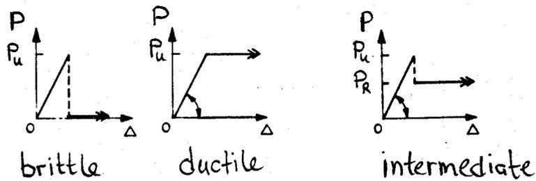
Figure C.2: Idealised load-displacement response of structural elements
