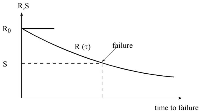
Figure B2: Load duration dependent strength under constant load
