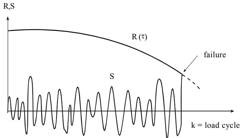
Figure B3: Fatigue fracture under cyclic loading
