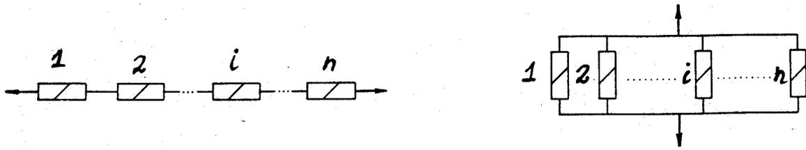
Figure C.1: Schematic representation of series and parallel systems
