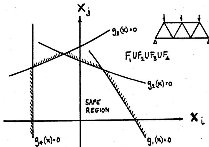
Figure C.6(a): Failure region as union of component failure events for series system
