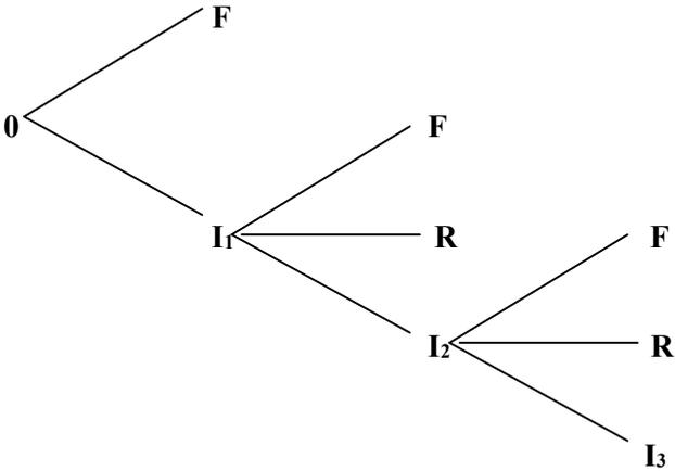
Figure B4: Event tree representation of an inspected component: R = Repair or maintenance action;
