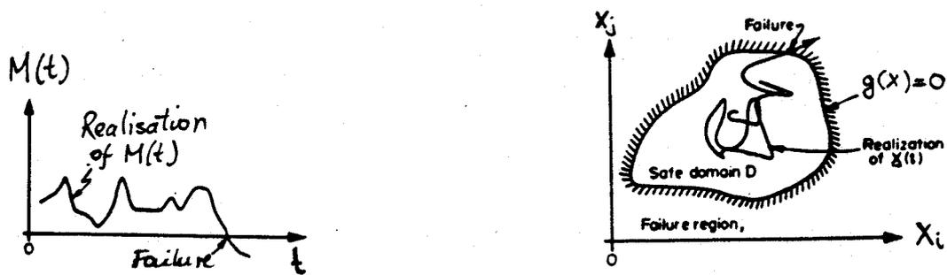
Figure C.12: Time-dependent safety margin and schematic representation of vector outcrossing
