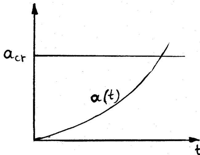
Figure C.10: Damage accumulation problem
