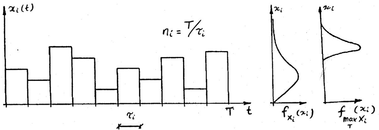
Figure C.11: Realization of an FBC process
