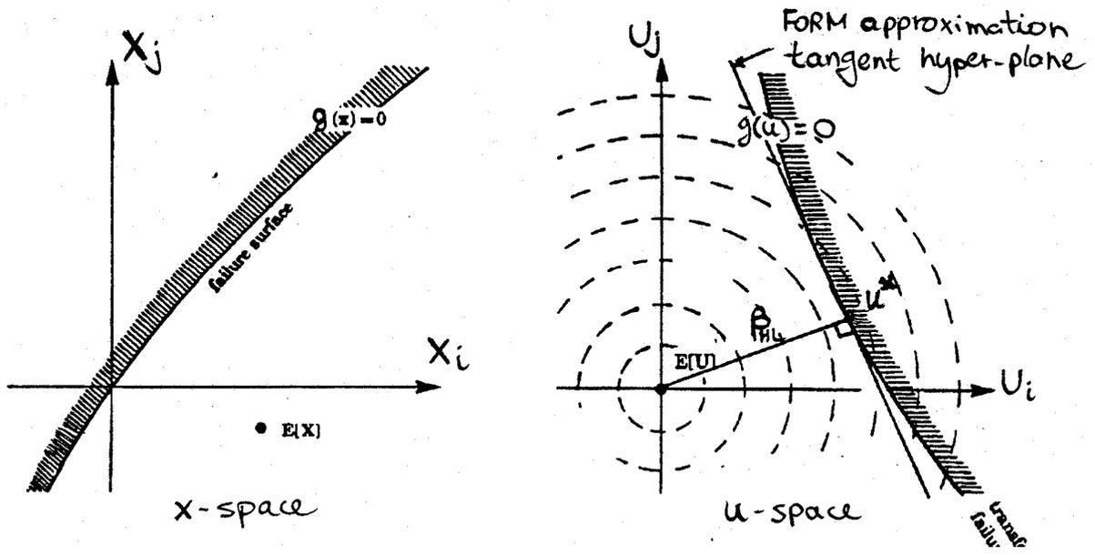
Figure C.5: Limit state surface in basic variable and standard normal space
