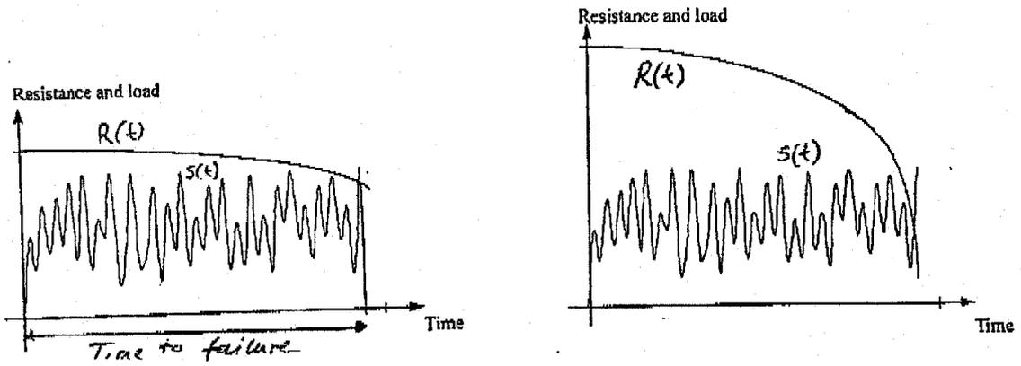
Figure C.8: Schematic representation of crossing problems
