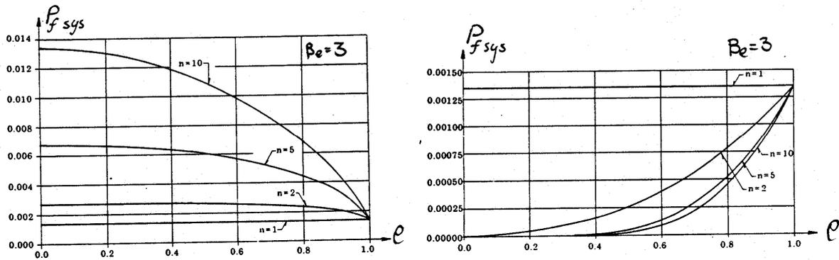
Figure C.3: Effect of element correlation and system size on failure probability
